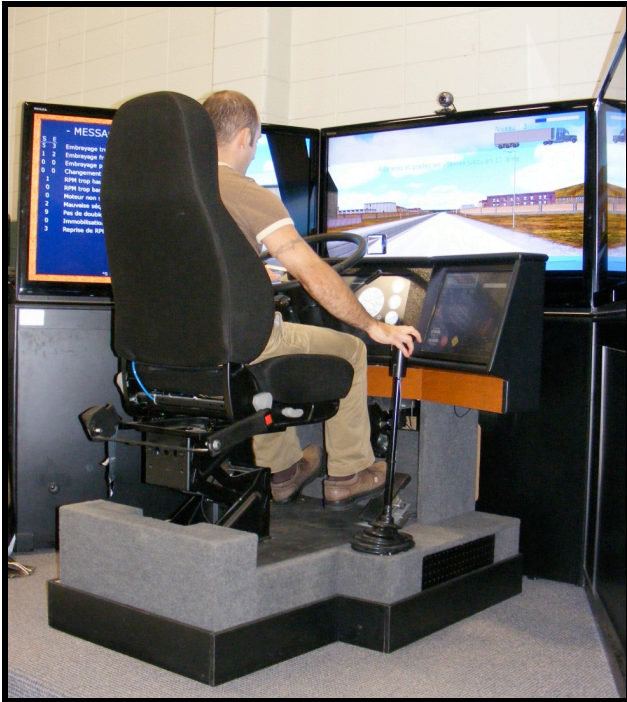
Figure 3. The VS600M is built with real truck components on a three degree of freedom motion / vibration platform and surround sound. Learners have a 180-degree forward field of view plus rear view mirrors and the manual shifter provides realistic force feedback and vibrations.
